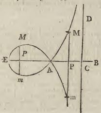
The portion between A and E is called a Nodus. If y be put =0, then the values of x are e, 0, —b. That is, the curve passes twice through A, or A is a punctum duplex, and it passes also through E as before. (1.)
